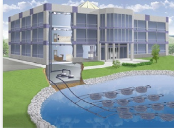
Figure 12: Geothermal Open Loop
